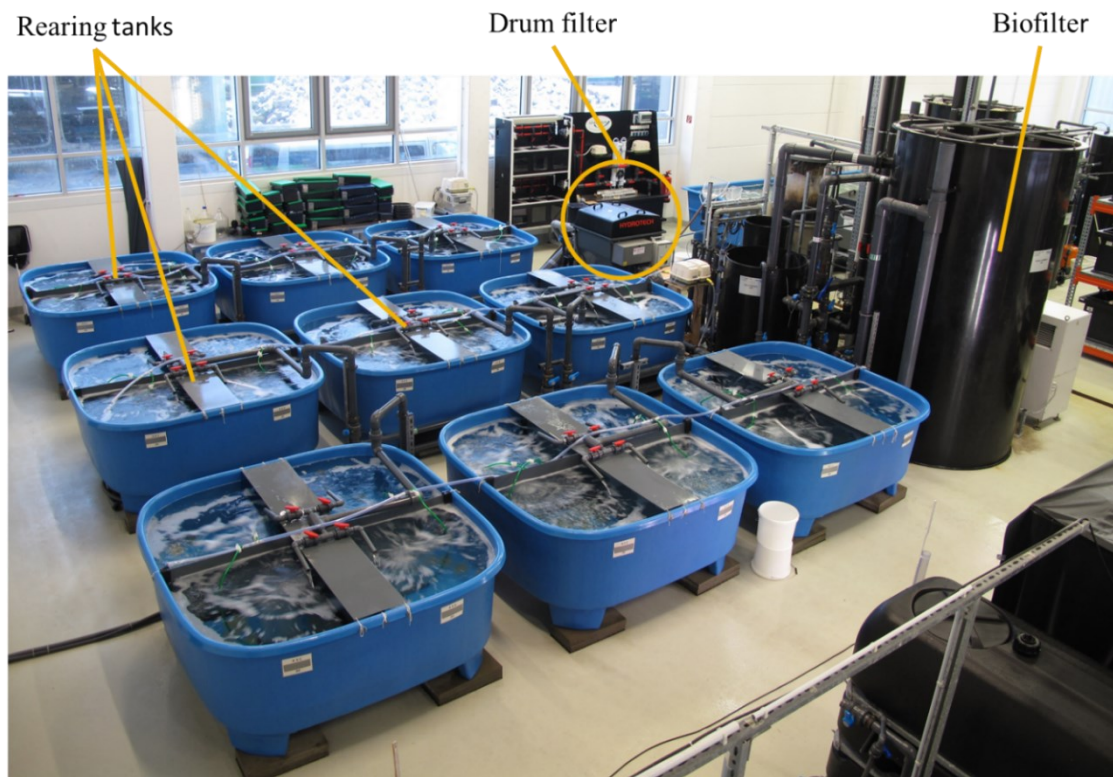
Figure 1.5. Image of a recirculating aquaculture system at the Center of Aquaculture Research of the Alfred-Wegener Institute, Helmholtz Centre for Polar and Marine Research in Bremerhaven, Germany. Orange lines indicate the rearing tanks (500 L), a drum filter and the biofilter unit.
